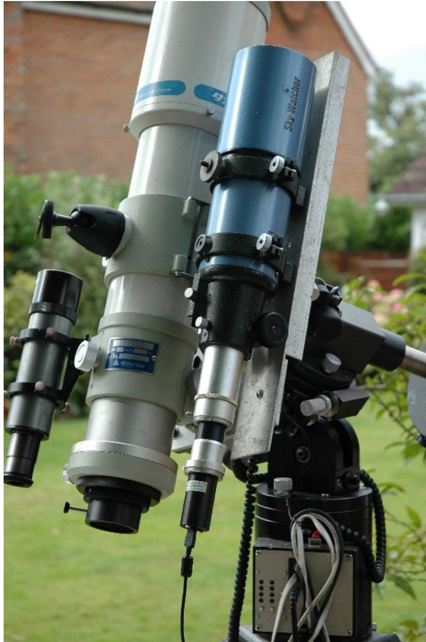
The Lodestar attached to an 80mm F5 guide 'scope
